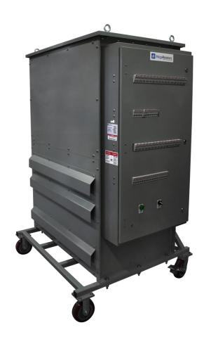
Installed in parallel with high-voltage equipment to release the charge from capacitors or batteries before maintenance. They can be used for rapid discharges or connected permanently for greater reliability and lower cost, balancing discharge time and energy loss during idle periods.
